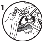
Gun locked (gun will not spray)
